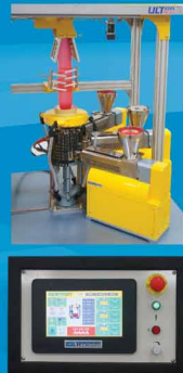
The Ultra Micro 3-Layers Co-Ex Blown Film line with 3 extruders
