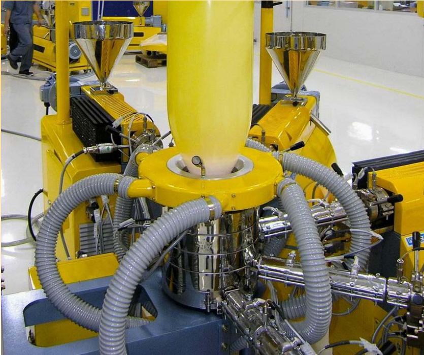
5-layer pancake die (LPD40-75/4) connected to 5 separate 20 mm extruders
